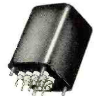
H-Type. Steel base cover deep-seal soldered into case. Terminals hermetically sealed. Ceramic bushings. Stud-mounted unit. Meets MIL-T-27 Specifications.
