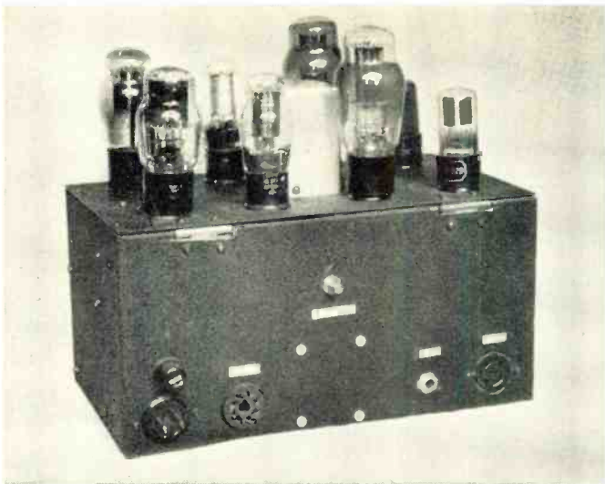
Over-all view of the high quality 50-watt amplifier. The power supply and main amplifier are housed in a 6" x 7" x 12" metal cabinet. All transformers, except the input coil, are mounted inside the cabinet. In later models the author added a row of cooling vents at the top and bottom of the housing.
